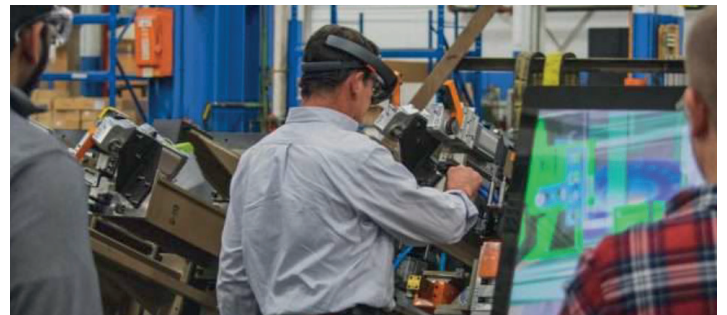
Ray Slowik pictured using a Microsoft HoloLens to compare physical and virtual part fixtures
