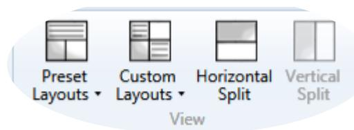
This allows the user to specify the number of panes and the layout of those panes. It also allows the layout and content (see Windows Area) to be saved as a named Layout. These layouts can be modified, re-saved and deleted as required.
