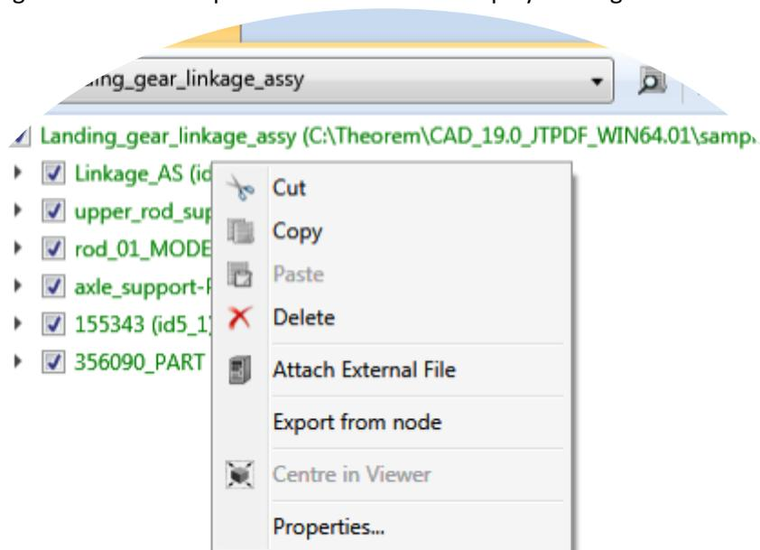
**Cut, Copy & Paste** lets the user move and copy existing nodes throughout the structure. Copying one part and pasting it under a different sub-assembly will use the original co-ordinate system of the part and then place it in the Structure relative to the sub-assembly co-ordinate system. Note that these features are only available with a DXN license.
