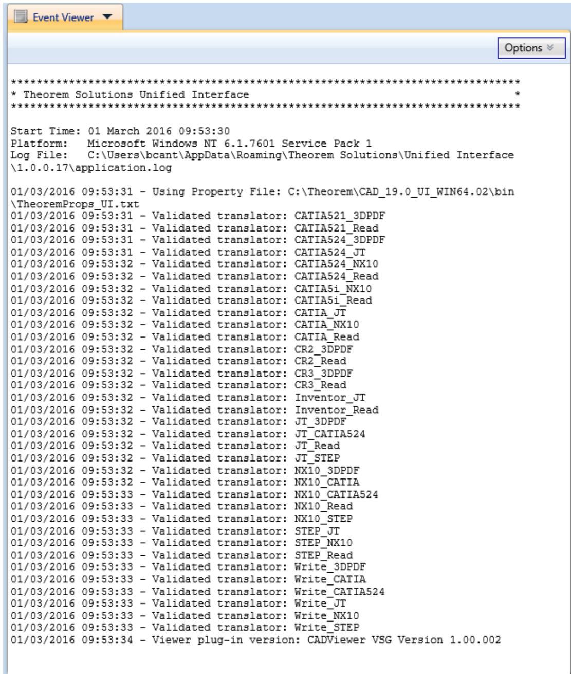
Options allows the user to switch line wrap on/off and gives the option to save the Event Viewer log to a specified location.
