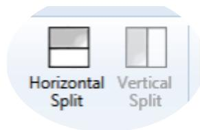
The Horizontal and Vertical Split buttons control whether the main split between the windows is vertical or horizontal. Note that in a Single Window View these options are not available.
