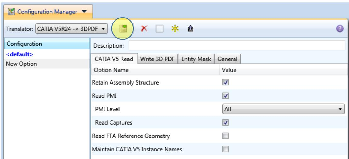
The Configuration Panel allows new configurations to be created based upon all available options within the selected application. Selecting the New Configuration icon will allow the user to change any option. For details on each option, refer to the Translator's User Guide or click the help icon in the Configuration Manager.
