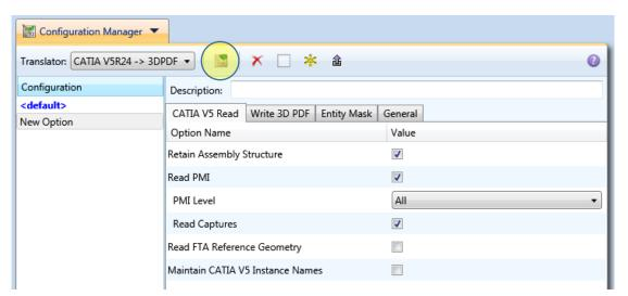
The Configuration Panel allows new configurations to be created based upon all available options within the selected application. Selecting the New Configuration icon will allow the user to change any option. For details on each option, refer to the Translator's User Guide or click the help icon 100 in the Configuration Manager.
