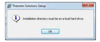
Therefore, the installation must be performed to a drive that is local to the machine itself. If you are attempting to install the software onto a network drive, then please refer to the configuration guide available from the following link:
