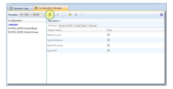
The Configuration Pane allows new configurations to be created based upon ALL available arguments within the Publish 3D application. Selecting the New Configuration icon will allow the user to change any Publish 3D argument.
