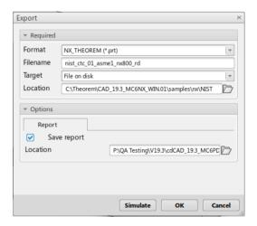
The "Save as types:" or "Format" selection should be set to NX\_THEOREM (\*.prt).
