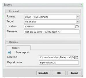
The "Save as types:" or "Format" selection should be set to CREO\_THEOREM (\*.prt or \*.asm).
