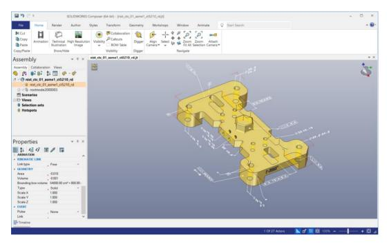
The diagram above shows an example of a JT file imported into the SWX Composer application showing the graphics in the main display area as well as the assembly structure and properties imported during the process.
